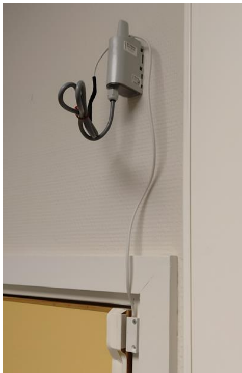
Figure 5.7: Dry Contacts sensor installed on the door of Room B237a
