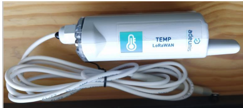
Figure 5.2: Adeunis TEMP: temperature sensor
