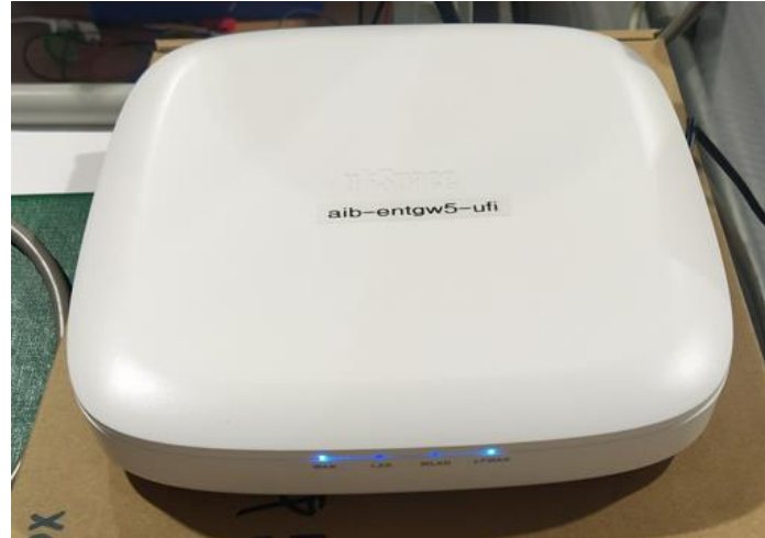
Figure 5.19: Indoor gateway UFISPACE PICO CELL "ENTERPRISE" installed in Process Hall
