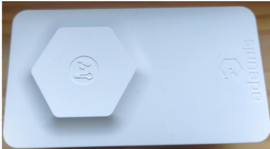
Figure 5.4: Adeunis COMFORT: temperature & relative humidity sensor
