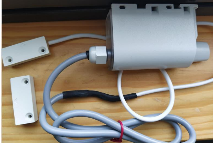
Figure 5.6: Adeunis Dry Contact sensor
